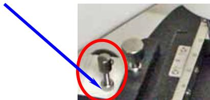
Do not worry about where it should be set since the 40X or the 100X objective can push inside itself and still not damage the objective. However, adjusting more than ¼ inch should be discouraged.
